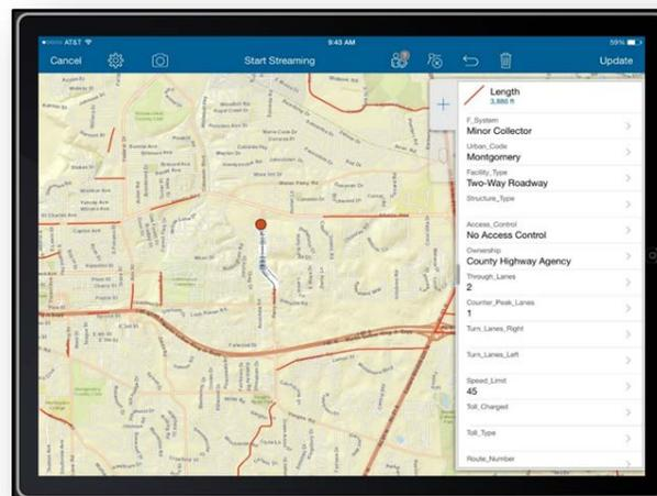
Figure 2. Illustration. Example of a data entry screen on an iPad from ALDOT's presentation.
